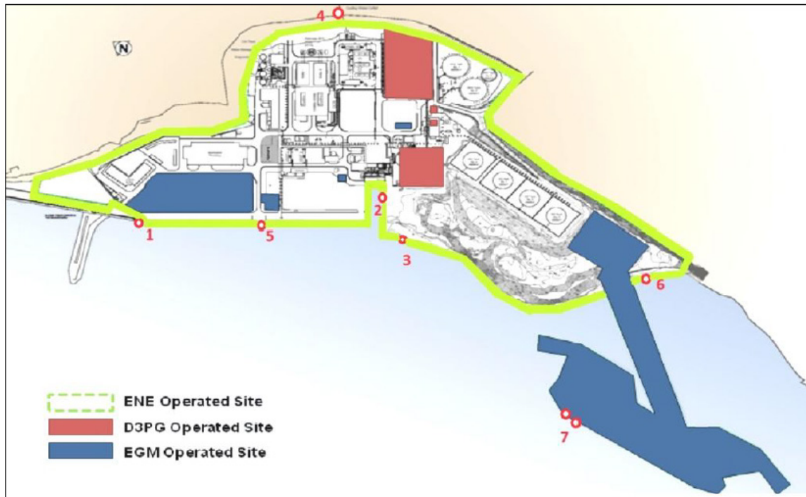
Figure 1: Effluent discharge points (1, 4, 6 and 7) pertaining to EGM's operations. Discharge Point 1: Runoff from EGM's Operated Site; Discharge Point 4: Cooling effluent discharged at il-Hofra z-Zghira; Discharge Point 6: Effluent from the Regassification Unit; Discharge Point 7: Effluent from the FSU. Discharge points 2, 3 and 5 do not relate to EGM's operations.
